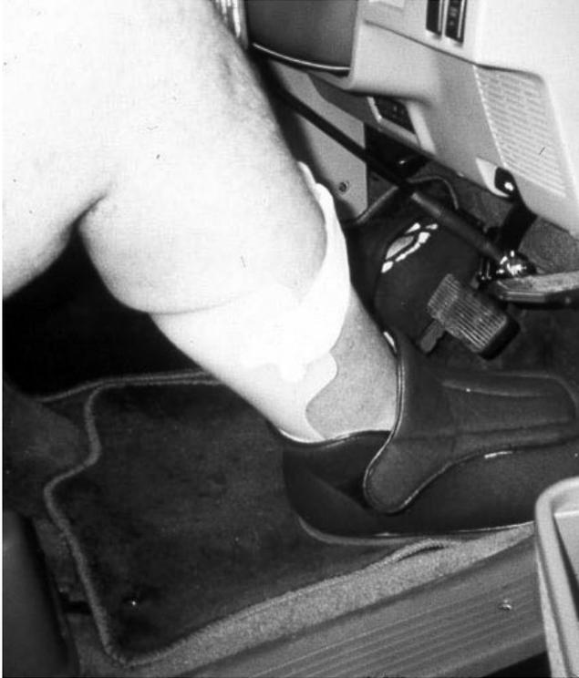
**Figure 43-4.** Foot positioning: Wearing an ankle-foot orthosis in a restricted space and weak thigh muscles make foot positioning difficult. This photograph shows the right accelerator pedal hinged out of the way for safety.
